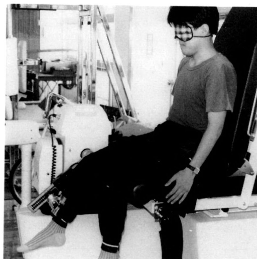
Fig. 1 Examination of reaction of hamstring muscles. The patients were instructed to react to the sudden forward movement of the input arm of a KIN-COM Dynamometer with contraction of the hamstrings.
